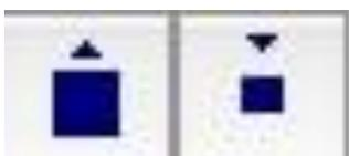
These buttons make the tube sizes bigger and smaller. For example, 380x380 to 390x390.
